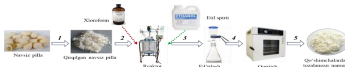
1 rasm. Navsiz pillani yog'-mumsimon va mineral qo'shimchalardan tozalash
