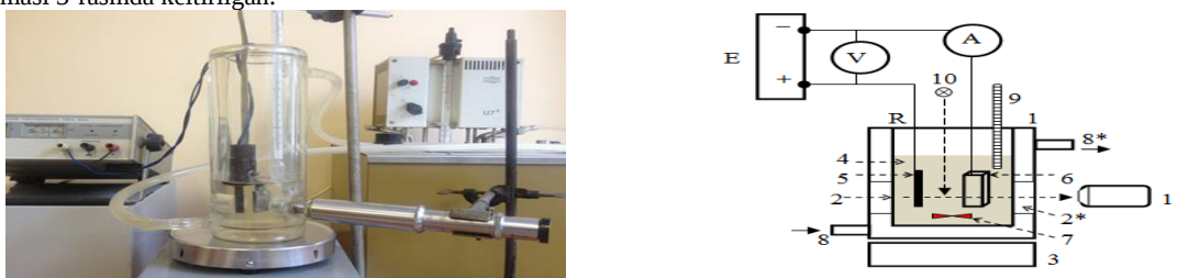
3-rasm. Takomillashtirilgan elektroliz qurilmasining fotosurati (a) va uning prinsipial chizmasi (b).
