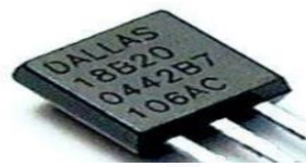
1-rasm. TO-92 korpusdagi DS18B20 sensor tasviri.
