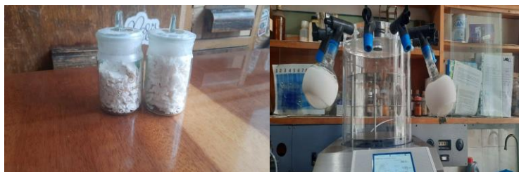
Rasm 4. Saccharomyces cerevisiae polipeptidining liofilizatsiya jarayoni
