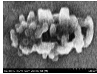
**2-rasm.**  $\sim 24 \pm 1^\circ\text{C}$  haroratda  $\text{C}_{70}$  mikrotomchisi bug'lanishi natijasida hosil bo'lgan  $\text{C}_{70}$  nanoagregatlarining SEM tasviri.
