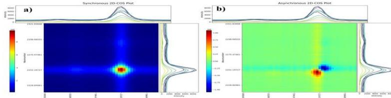
Figure 2. Synchronous (a) and asynchronous (b) 2D Raman correlation spectra of the ACN-DMSO mixture were constructed from the selected concentration range from 1 to 0.05 mole fraction.
