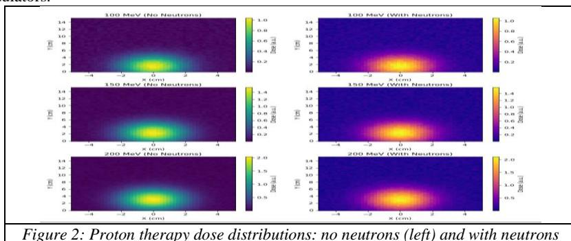
Figure 2: Proton therapy dose distributions: no neutrons (left) and with neutrons (right)
