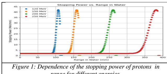
Figure 1: Dependence of the stopping power of protons in range for different energies.
