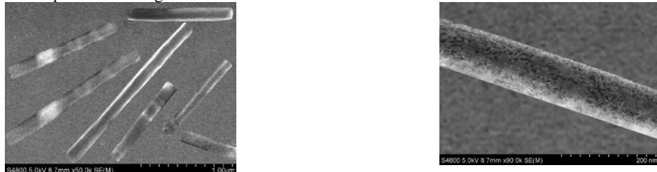
**5-rasm.**  $\text{C}_{70}$  molekular eritmasining bug'langan tomchisida ( $T \approx 36^\circ\text{C}$ ) sintez qilingan nanoviskerlarning SEM tasviri
